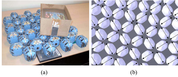
Fig. 3. An intelligent conveyor surface constructed from ATRON modules. (a) Conveyor surface build from ATRON modules moving a box. (b) Screen shot from the ATRON simulator. The arrows show how the individual modules can move objects. This high degree of flexibility makes it possible to move objects in any direction and to rotate objects.
