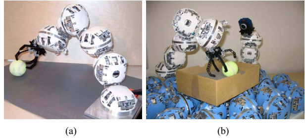
Fig. 4. (a) Three degree of freedom robotic arm (first two joints are locked), with a gripper, reaching for a yellow ball. The gripper is held by one male connector and actuated, via strings, with the other male connector on the same hemisphere. (b) Manipulation system assembled from ATRON modules. The box rest on an conveyor surface, in the back a small robot arm is equipped with a camera, in the front a robot arm with a gripper (note: conceptual setup only).
