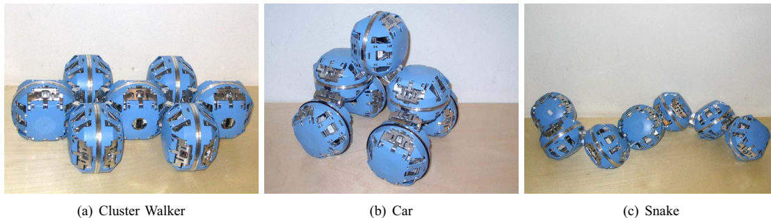
Fig. 2. Different configurations all consisting of 7 ATRON modules. (a) configuration capable of performing cluster walk. (b) four wheeled car. (c) snake configuration. The robot is able to autonomously reconfigure between any of these configurations that have different locomotion characteristics.
