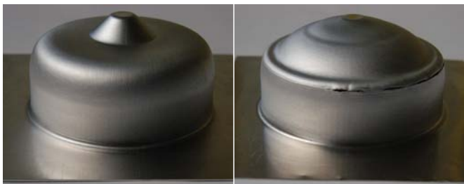
Fig. 6 Geometry after 4 stages of forming (left DDDU and right DUDD).
