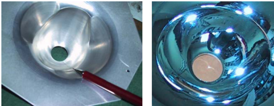
Fig. 11 Left: prototype of headlight reflector, right: reflector after surface treatment [26]
