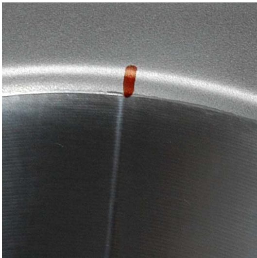
Fig. 15 Inner surface of cone made with profile tool path
