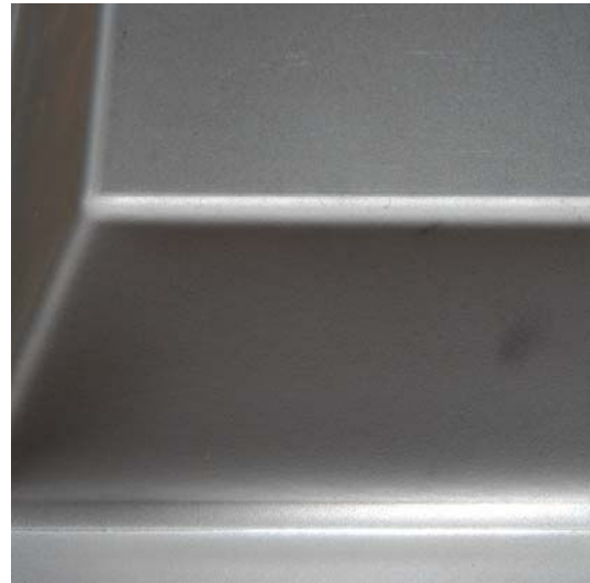
Fig. 10 Outer surface of pyramid made with helical tool path
