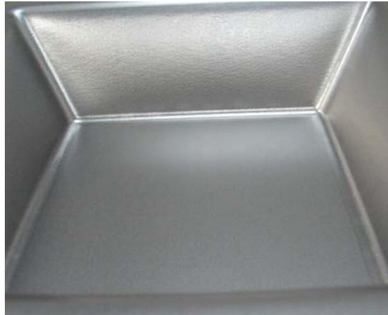
Figure 10: Pyramid formed using a dummy sheet with dry friction
