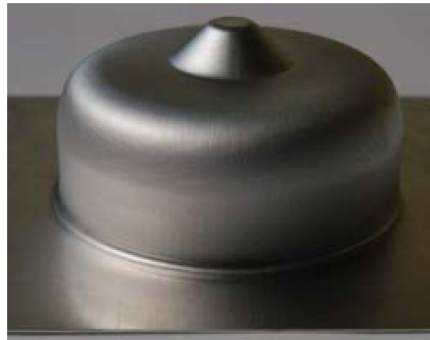
Fig. 40 Cup with 90^\circ walls formed in four stages [46]
