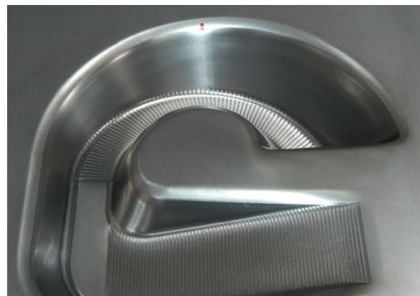
Fig. 21 Muffler made with helical tool path
