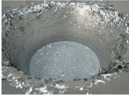
Figure 16: Severe galling in forming of hyperboloid in 2 mm AA1050 H111
