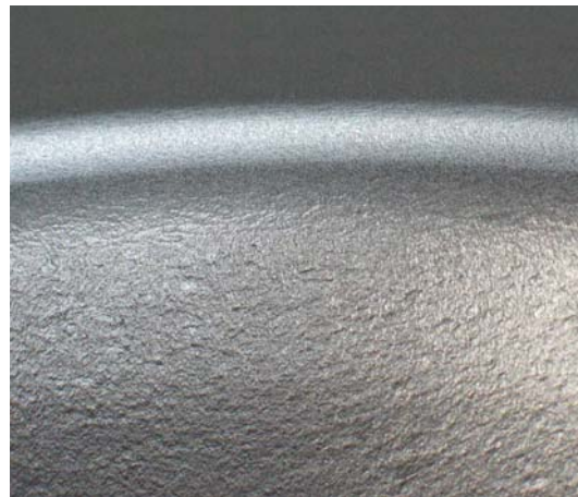
Figure 12: Surface of hyperboloid using a dummy sheet with dry friction
