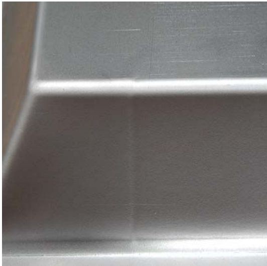
Fig. 9 Outer surface of pyramid made with profile tool path
