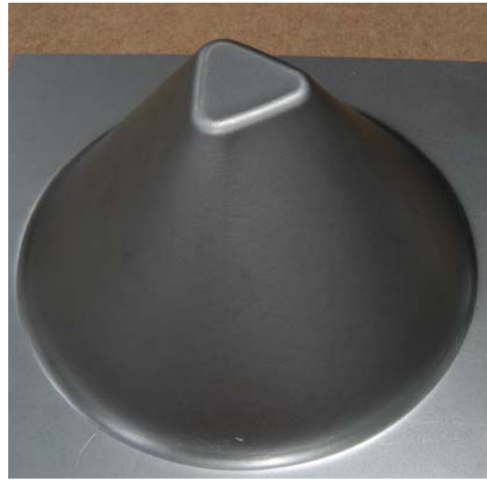
Fig. 14 Outer surface of cone made with helical tool path
