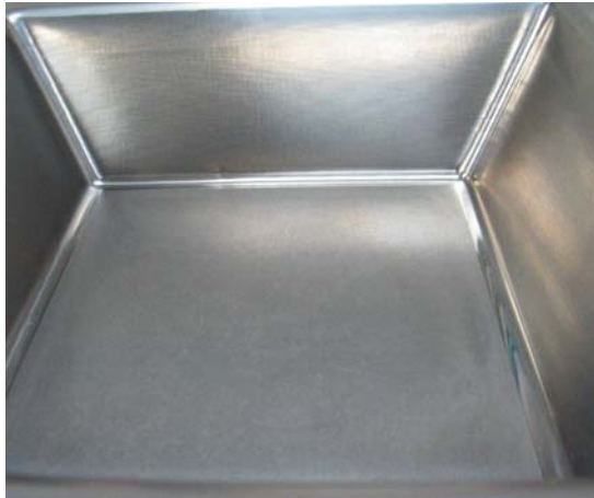
Figure 9: Pyramid formed with traditional SPIF
