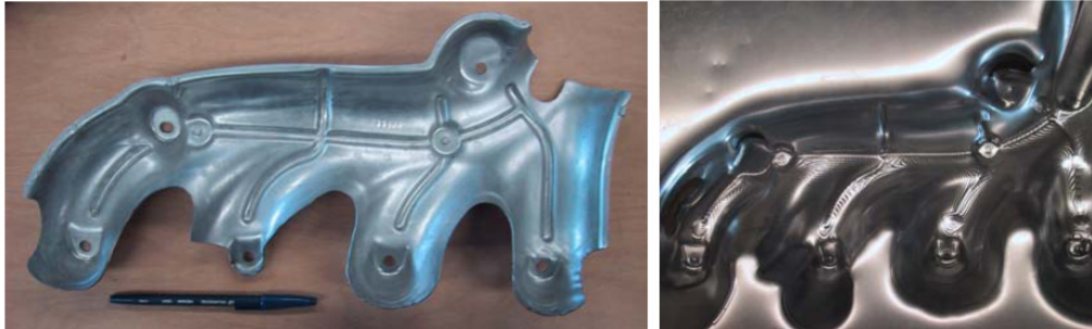
Fig. 10 Left: original manifold heat shield, right: prototype produced by SPIF [17]
