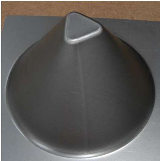
Fig. 13 Outer surface of cone made with profile tool path
