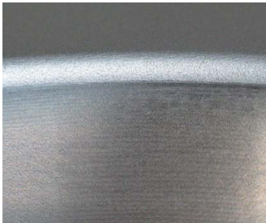
Figure 11: Surface of hyperboloid formed with traditional SPIF
