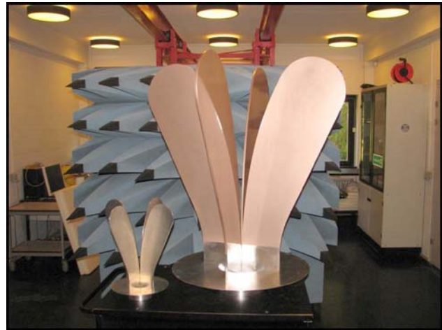
Figure 2 - The manufactured 1-3 GHz and 0.4-1.2 GHz dual-polarized probes.
