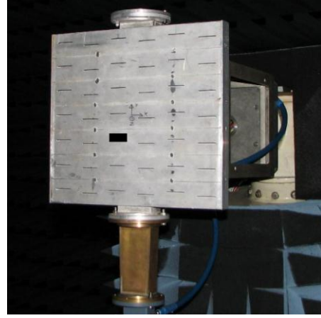
Figure 1 – The 6 by 7 slotted waveguide array in the DTU-ESA Spherical Near-Field Antenna Test Facility.
