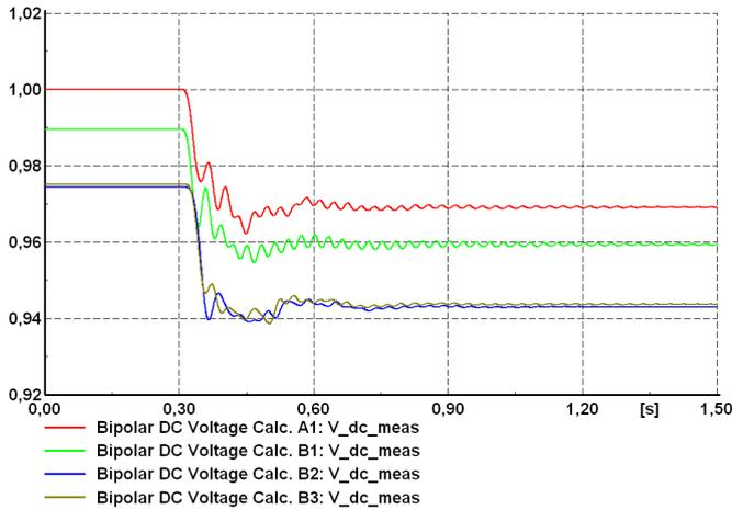
Figure 11: DC current based control - DC voltage.
