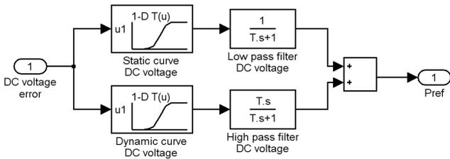
Figure 4: Block diagram of improved undead-band controller.
