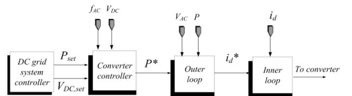
Figure 1: Overall block diagram for undead-band control.
