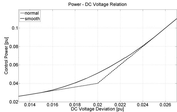
Figure 3: Original characteristic curve and smooth curve.
