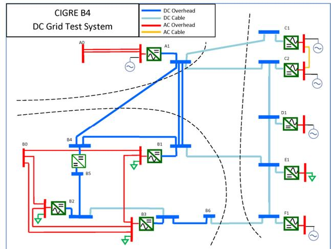
Figure 6: CIGRE B4 DC grid test system.
