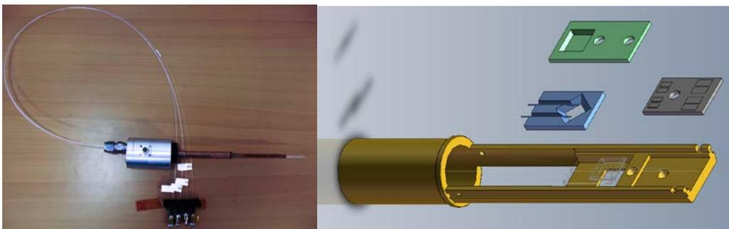
**Figure 1.** (Left) Photograph of the specimen holder shown without a tip for ease of visualization [7]. (Right) Schematic drawing of the specimen holder tip, including the mirror chip (blue), the heater (green) and the contact pad (grey).
