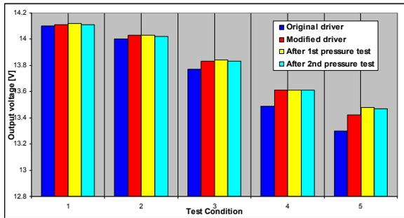
**Fig. 9.** Modified driver, before pressurization (blue), after first pressurization (red) and after second pressurization (green)
