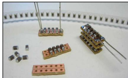
Fig. 4. Stacked ceramic capacitors for electrolytic replacement
