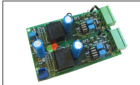
Fig. 3. Original in-house IGBT gate driver
