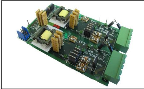
Fig. 6. Modified IGBT gate driver
