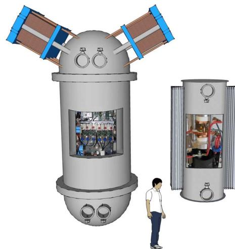
**Fig. 1.** Representative case of a Today's subsea converter (left) and of a pressure compensated converter (right).
