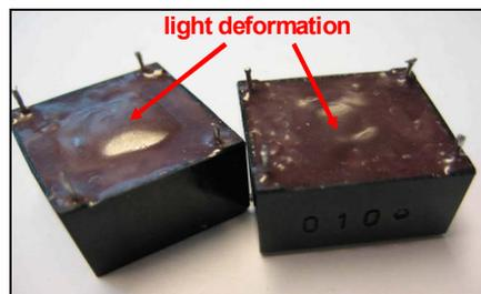
Fig. 5. Examples of damages due to exposure to high pressure hydrostatic environment followed by abrupt depressurization
