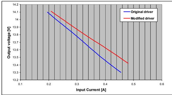
**Fig. 8.** Original (blue) and modified (red) drivers, output voltage as function of current drawn at input
