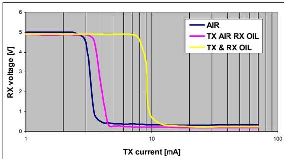
Fig. 7. HFBR-0501 threshold comparison in air and dielectric liquid, logarithmic scale
