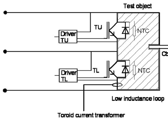
Fig. 2. IGBT phase-leg (test object)
