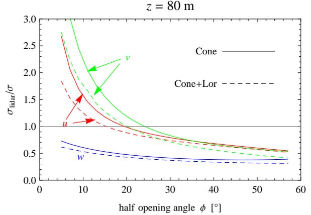
Figure 3: The sensitivity of the systematic errors to  $\phi$  at  $z = 80$  m. The solid line shows only cone averaging and the dotted line shows the averaging due to cone and  $\varphi$ , where  $\varphi$  is modelled using Lorentzian
