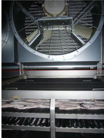
Figure 1. Inside the CBC-cooler, fillets are laid down on the skin and superchilled with blast and contact cooling.
