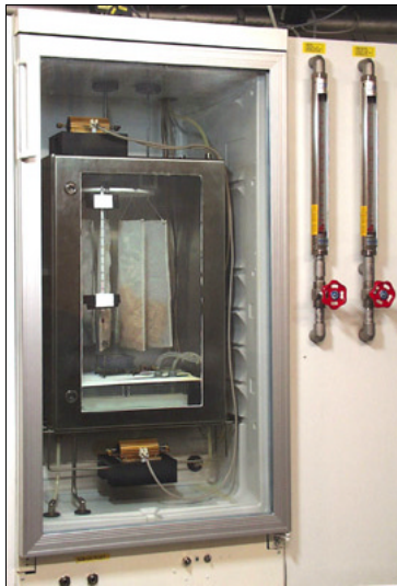
Figure 4.3. Climate chamber exclusively developed for measurements at elevated temperature.
