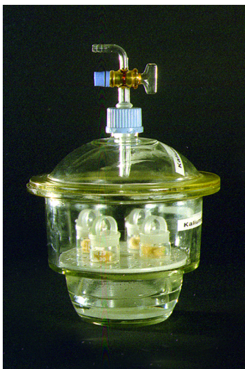
Figure 3.1. Desiccator containing a saturated salt solution and small samples in glass containers.
