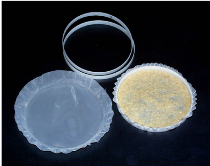
Figure 5.2. Sample container for pressure plate and pressure membrane apparatus. Exclusively for wood and plant fibres.
