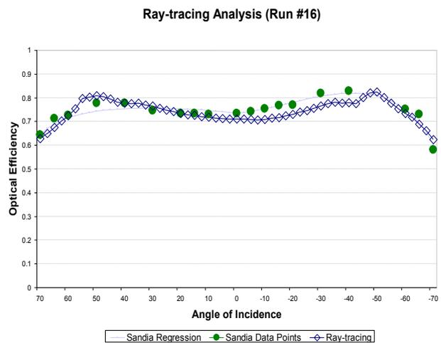
Fig. 10: Optical efficiency plots of ray-tracing analysis (Run #16)
