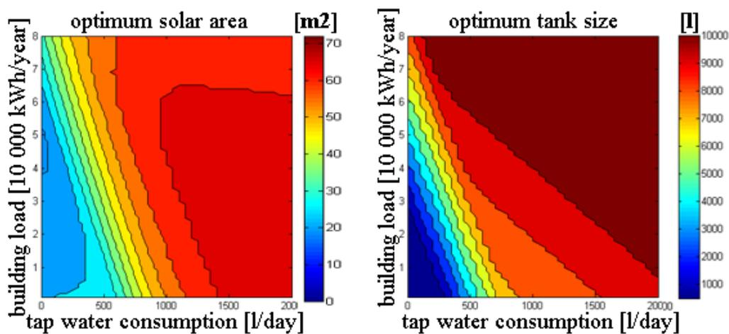
Fig. 4. Optimum for building load and tap water consumption. Left: Collector area Right: Tank size
