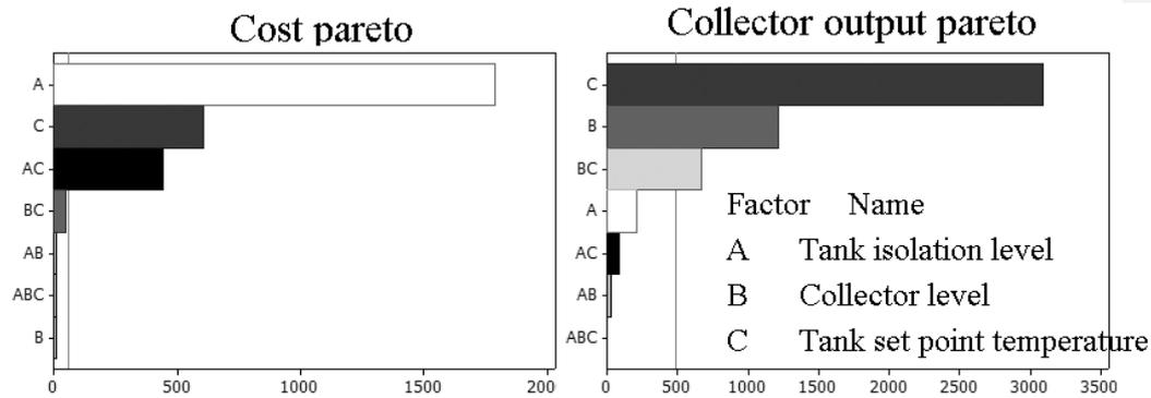
Fig. 9. Cost-dependence variables affected by tank set-point temperature.
