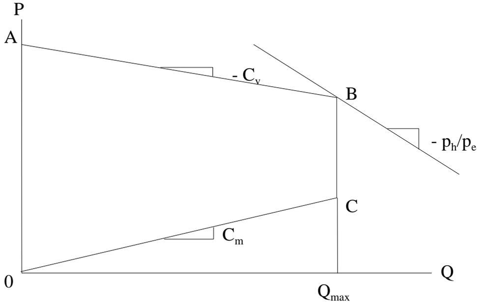
**Figure 1. Production possibilities for an extraction condensing plant.**
