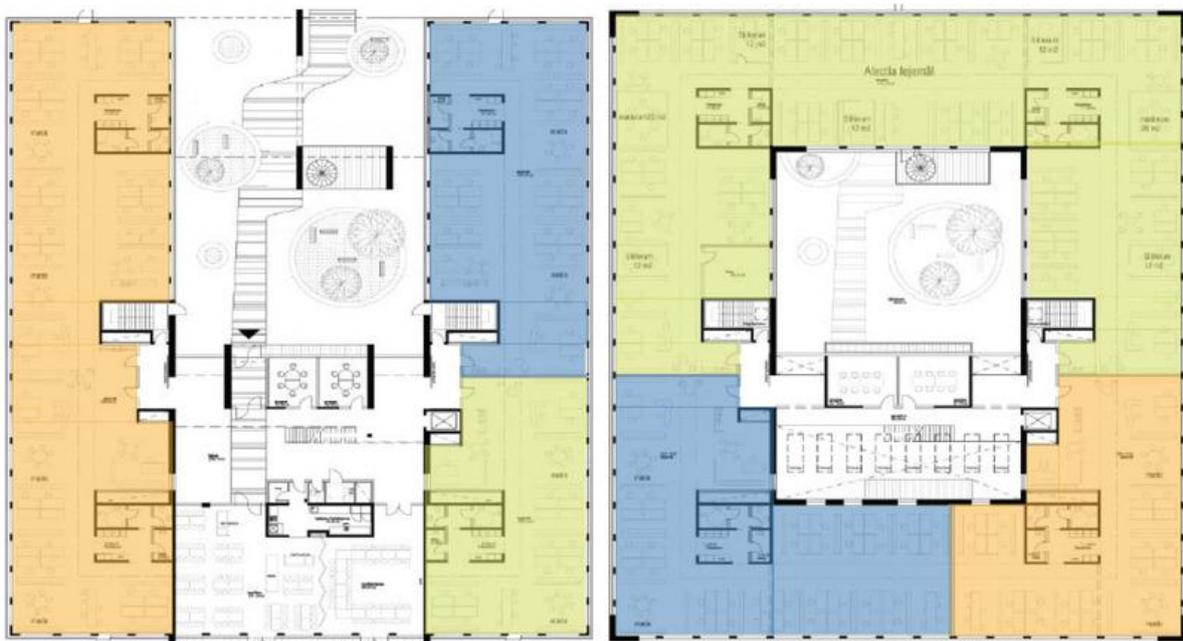
*Figure 2 Plan drawings for Company House III in Kolding, Denmark. The colours indicate the various areas for lease and the white areas are common, shared facilities like arrivals area, canteen and meeting rooms.*
