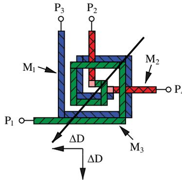
**Figure 5.** Illustration of offset broadband coupled spiral transformer configuration for EM simulation based optimization. The offset distance is represented by  $\Delta D$  and the port designation follows that of a standard coupled line.
