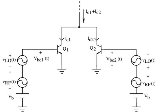
**Figure 1.** Simplified schematic of balanced sub-harmonic mixer configuration.
