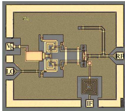
**Figure 7.** Microphotograph of fabricated SHM with miniature spiral type Marchand balun.
