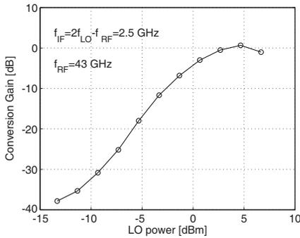
**Figure 8.** Measured conversion gain versus LO power.
