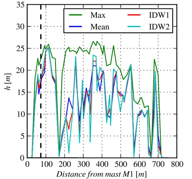
**Figure 5:** Forest height estimations  $h$  on the  $200 \times 200$  fine forest height grid from the different interpolation methods of the point cloud. IDW1 and IDW2 denotes the inverse distance weighting method with for a weighting exponent of respectively  $p = 1$  and  $p = 2$ . The dashed line indicate the position of mast M2.
