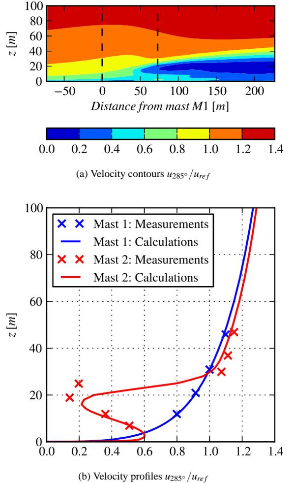
**Figure 7:** (a) Calculated velocity contours for the transect shown in Fig. 5 for the max method (the dashed lines indicate the positions of the masts) and (b) comparison of measured and calculated wind velocities at mast M1 (blue curve) and mast M2 (red curve) locations (see Table 1) for the  $\theta = 285^\circ$  flow direction. The reference velocity  $u_{ref}$  is taken at mast M1 at  $z_{ref} = 30.9m$  for both, wind measurements and calculations.
