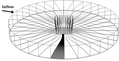
**Figure 4:** Layout of the multiblock computational grid.
