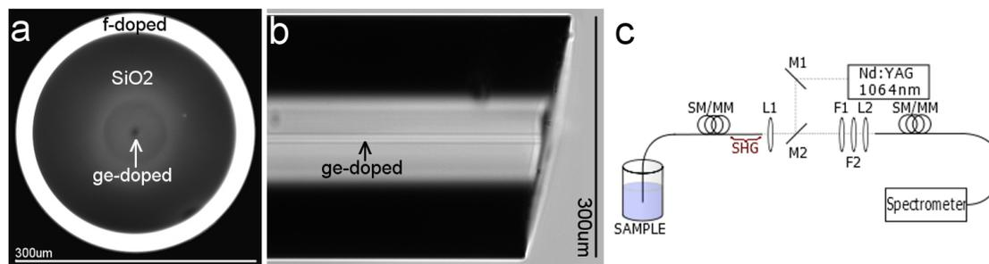
Fig. 1. (a) Cross-section of the dual-core fiber; (b) Angle-cleaved tip (about  $11^\circ$ ) on the sample side; (c) Schematic illustration of the setup: M1,2 are mirrors (M2 is dichroic), L1,2 are 10x focusing lenses, F1 is a dual notch filter, F2 is a KG5 glass filter. The double-core fiber is indicated as SM/MM. The spectrometer is connected to a computer (not shown).
