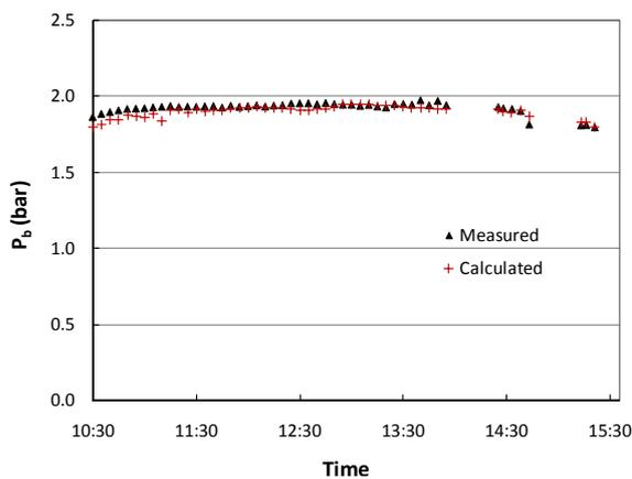
Fig.4 Measured and calculated pressure of the bottom of the solar collector loop during stagnation, September 1, 2009
