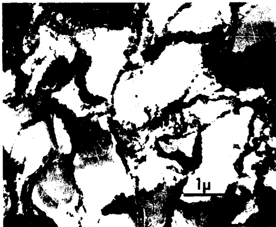
FIG. 5.—Transverse section of an extruded rod manufactured from Al MD 105 containing 8 wt.-% \text{Al}_2\text{O}_3 Cl. Billet temperature 330°C. Extrusion ratio 15:1.
