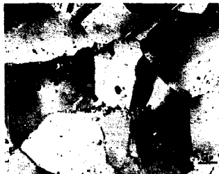
Fig. 1—Microstructure of an extruded aluminum aluminum-oxide product containing 0.2 wt pct of aluminum oxide (Al ND 13), heat treated for 6 hr at 500°C after extrusion. Transversal section.
