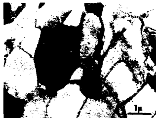
Fig. 3—Microstructure of 99.998 pct Al reduced 80 pct in area by drawing and heat treated for 12 hr at 140°C. Longitudinal section.
