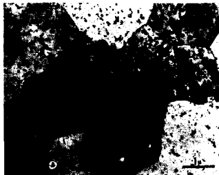
Fig. 2—Microstructure of an extruded aluminum aluminum-oxide product containing 1.2 wt pct of aluminum oxide (Al R 400), heat treated for 12 hr at 635°C after extrusion. Transversal section.
