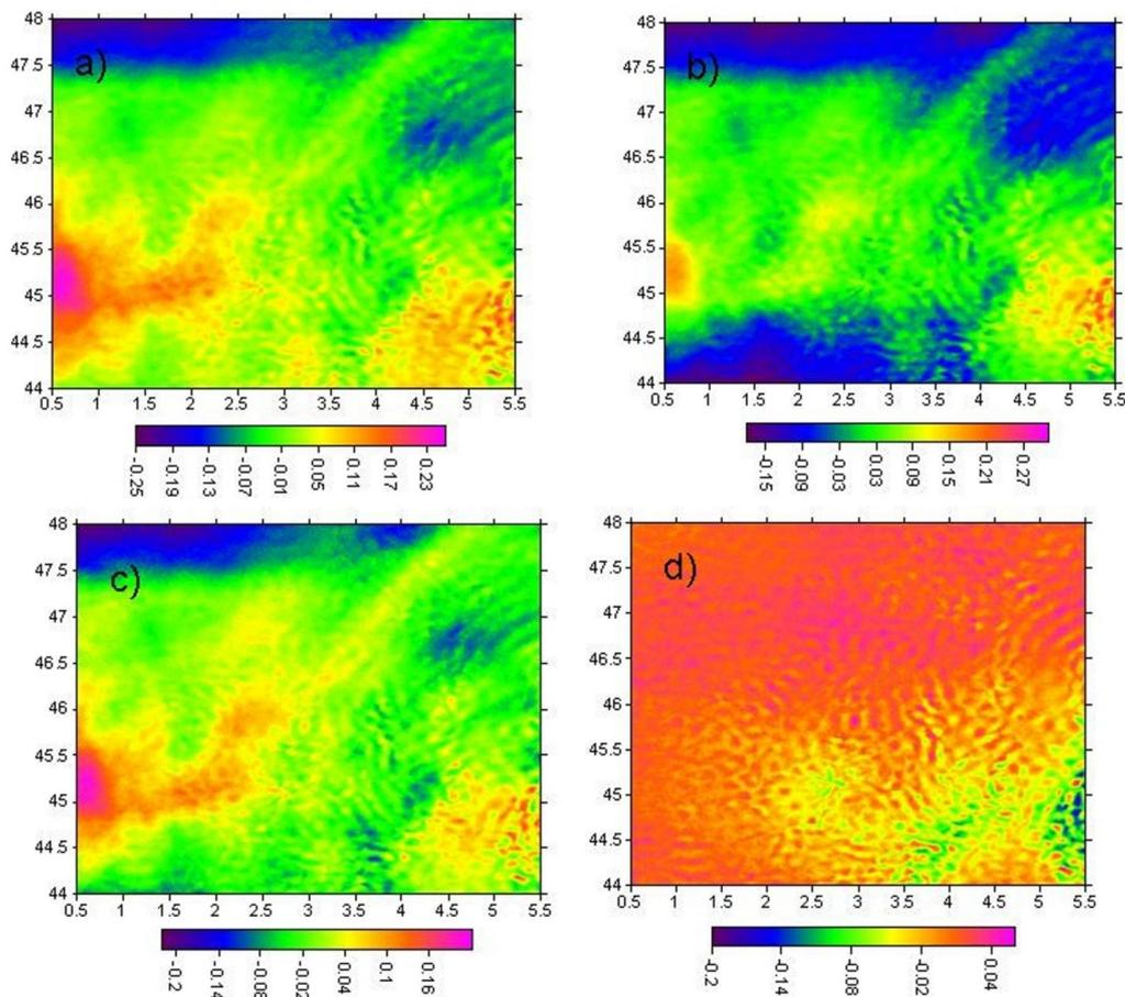
Figure 8. Comparison of the quasi-geoid models with EGM2008 quasi-geoid heights. a)  $\text{FFT}^{(1)}$  minus EGM2008; b)  $\text{FFT}^{(2)}$  minus EGM2008; c) LSC minus EGM2008; d) LSMS minus EGM2008. Unit is in metre
