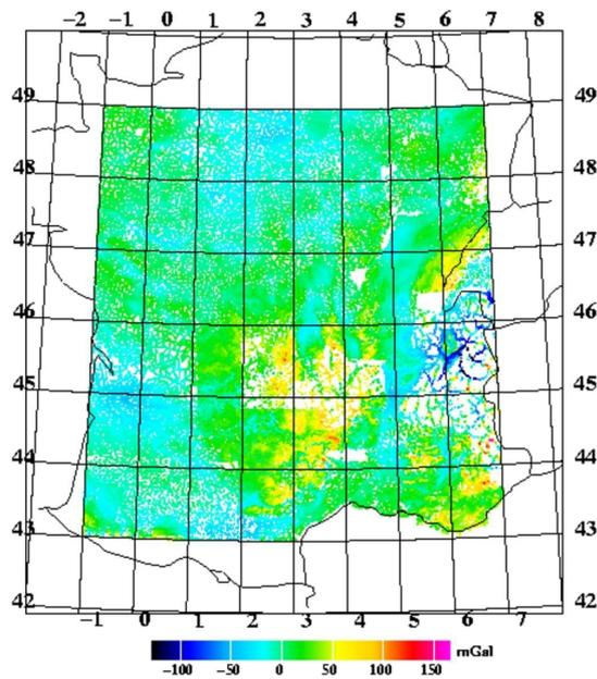
Figure 2. The selected 59097 surface gravity anomalies at  $0.02^\circ \times 0.025^\circ$  resolution (pixel binning to approx. 2 km resolution) used as identical input for the implementation of all three quasi-geoid determination methods
