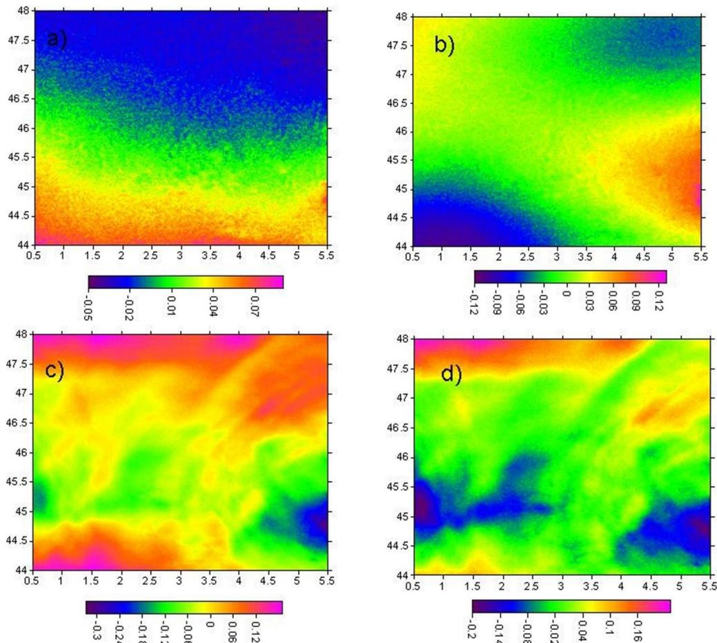
Figure 7. Inter-comparison of the quasi-geoid models. a) FFT<sup>(1)</sup> minus LSC; b) FFT<sup>(2)</sup> minus LSC; c) LSMS minus FFT<sup>(2)</sup>; f) LSMS minus LSC. Unit is in metre
