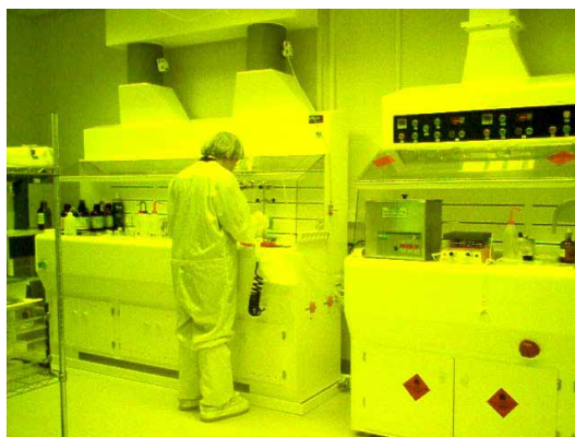
Fig. 1. A typical photolithography room illuminated by a yellow fluorescent light tube [2].
