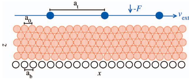
FIG. 1. A sketch of the model with the rigid top (solid circles) and bottom (open) crystalline sliders (of lattice spacing  $a_t$  and  $a_b$ , respectively), the former moving at externally imposed  $x$ -velocity  $v_{\text{ext}}$ . One or more solid lubricant layers (shaded) of rest equilibrium spacing  $a_0$  are confined in between.
