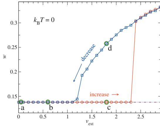
FIG. 10. The average velocity ratio  $w = \overline{v_{cm,x}}/v_{ext}$  as a function of the adiabatically increased (circles) or decreased (squares) top-layer velocity  $v_{ext}$ . The model parameters are the same as in Fig. 8, but with no thermal effects ( $k_B T = 0$ ).
