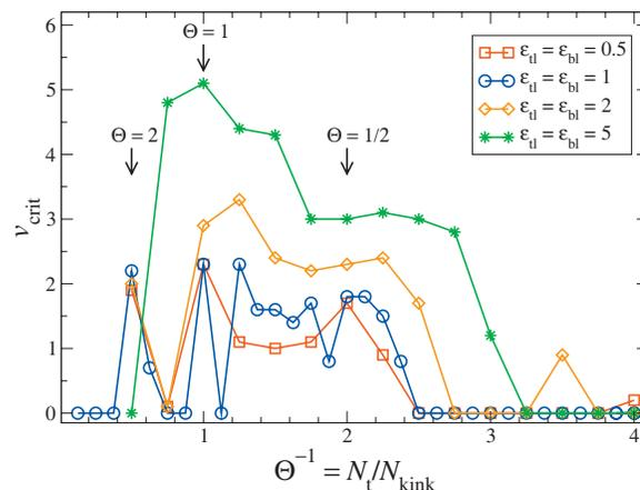
FIG. 5. Variation of the plateau boundary velocity  $v_{\text{crit}}$  as a function of the kink coverage  $\Theta^{-1} = N_t/N_{\text{kink}}$  for a lubricant monolayer showing different interaction energies with the substrates. Simulations are carried out with the same conditions as in Fig. 4, but with varied  $\epsilon_{\text{il}} = \epsilon_{\text{bl}}$ , (but unchanged interparticle interaction  $\epsilon_{\text{ll}} = \epsilon$ ).
