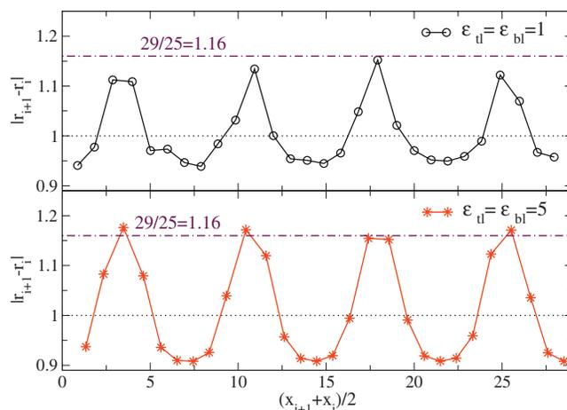
FIG. 6. Snapshot of the dynamically pinned state of the 2D lubricant, showing the bond lengths as a function of the bond horizontal position along the slider. Shorter bonds  $\approx a_b$  identify kink regions, while longer bonds  $\approx 1.16a_b$  belong to in-register regions. Larger interaction with the substrates  $\epsilon_{\text{il}} = \epsilon_{\text{bl}} > 1$  favors the commensurate in-register region.
