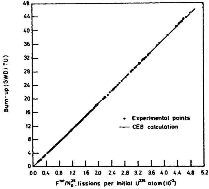
Fig. 5.4. a. Fuel burn-up versus total accumulated fissions.
