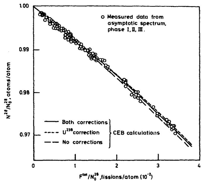
Fig. 5.4.d.  $U^{238}$  concentration versus accumulated fissions.
