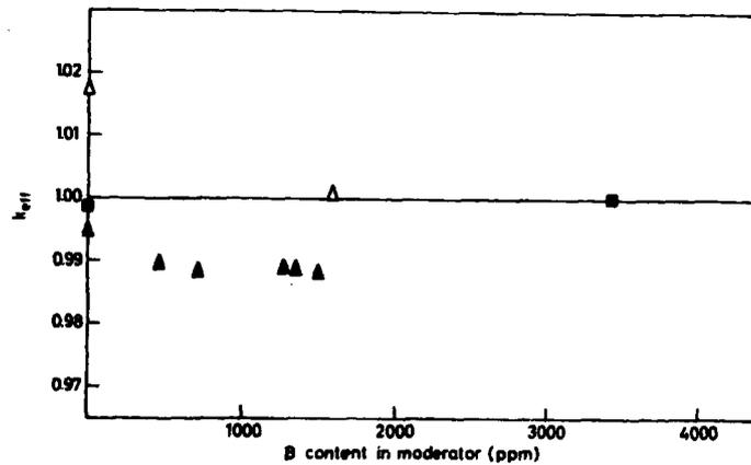
Fig. 6.2.f. Calculated  $k_{eff}$  versus moderator boron content.
