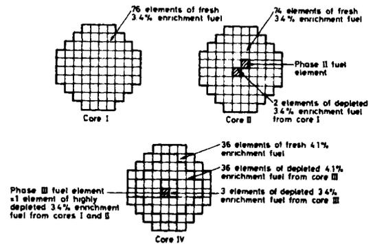
Fig. 5.1.b. Yankee cores I, II, and IV.
