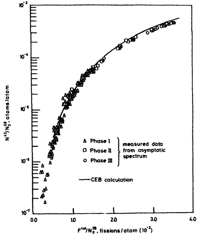
Fig. 5.4.h.  $\text{Pu}^{242}$  concentrations versus accumulated fissions.
