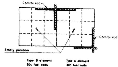
Fig. 5.1.a. Yankee fuel element cross section.
