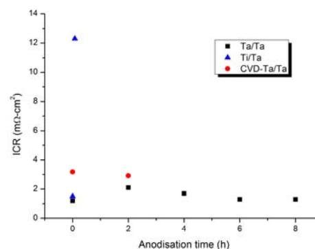
**Figure 2:** Interfacial contact resistance of tantalum, tantalum coated and titanium in contact with tantalum as function of anodisation time. Anodisations were performed at 130 °C, 2 V in 85% H<sub>3</sub>PO<sub>4</sub>.
