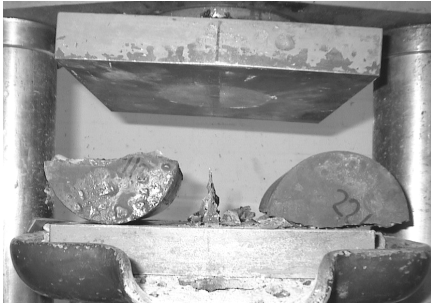
Figure 5.16 The outcome of a split cylinder test when performed on an early age concrete. Ordinary normal strength concrete specimen, 12 hours old, diameter 100 mm, length 200 mm, width of loading strip 10 mm.
