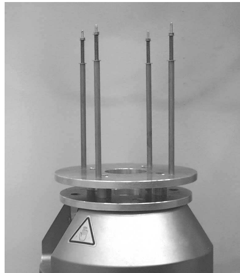
Figure 7.12 The self-weight is eliminated by springs which support the concrete and reinforcement self-weight. The springs are so soft that their reaction imposed on the specimen does not change during experiment.
