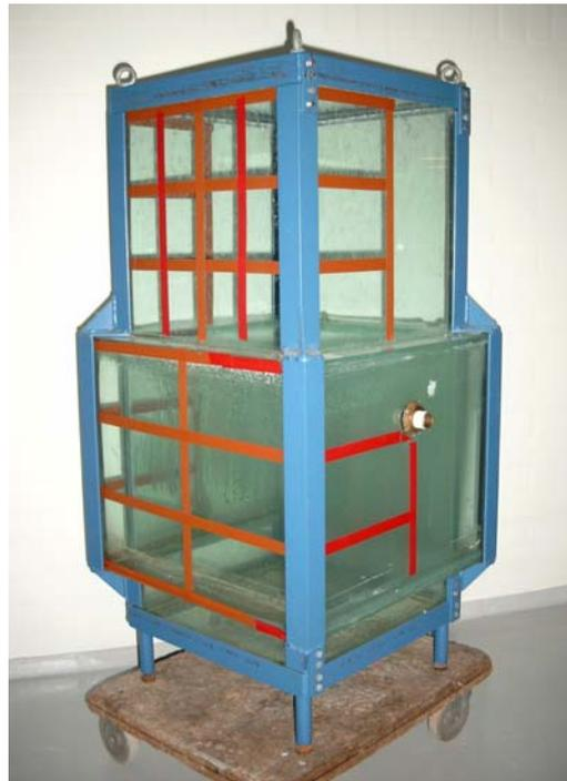
Figure 5-9: Glass model of mantle tank.
