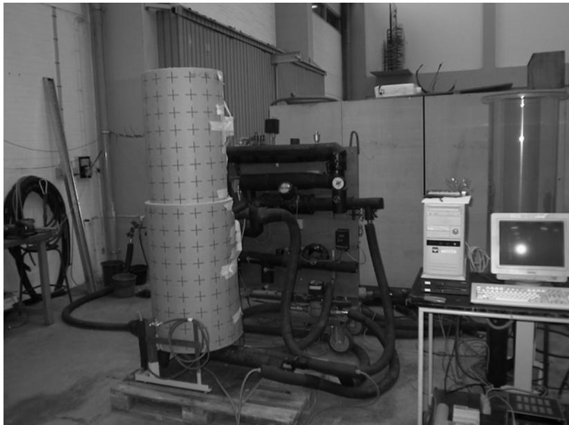
**Figure 3-1: Experimental set-up in the heat storage test facility.**
