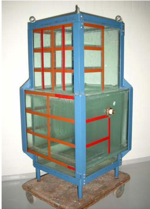
Figure 3-5: Glass model of the mantle tank.
