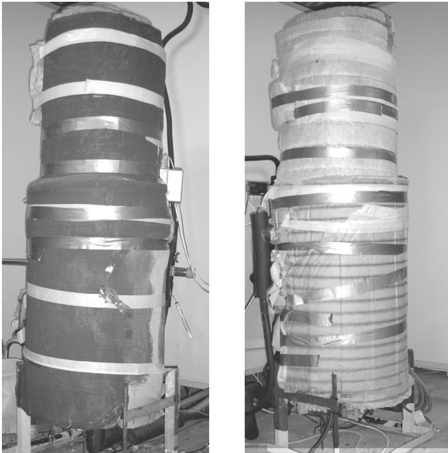
**Figure 4-46: Left: Heat storage in system with lower mantle inlet. Right: Heat storage in system with top mantle inlet.**
