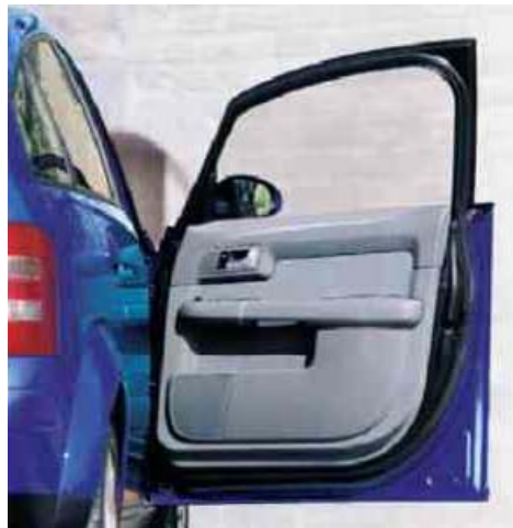
FIGURE 2.22. A side door liner of an Audi A2 based on a plant fibre composite material. From N-fibrebase (other examples of applications can be seen in this internet database).
