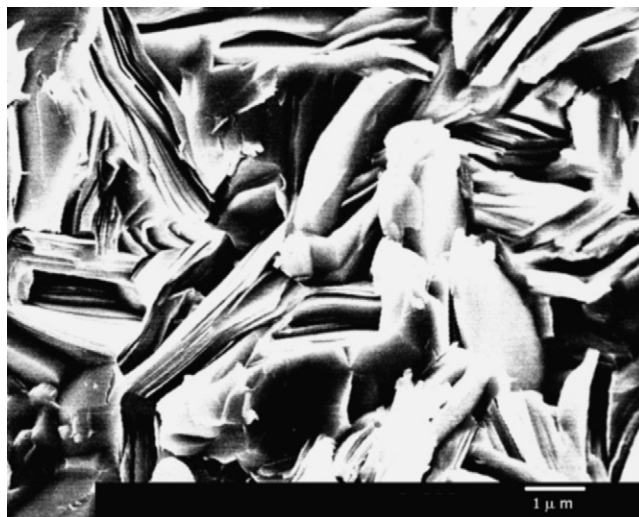
Fig. 3. SEM photograph of the fractured surfaces of the x=0.05 sample.
