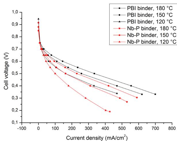
Figure 1: Polarisation curve for electrodes. Both electrodes had a Pt loading of 0.7 mg/cm<sup>2</sup>. One electrode had a Nb-P loading of 1.2 mg/cm<sup>2</sup> and the other had a PBI loading of 0.14 mg/cm<sup>2</sup>.
