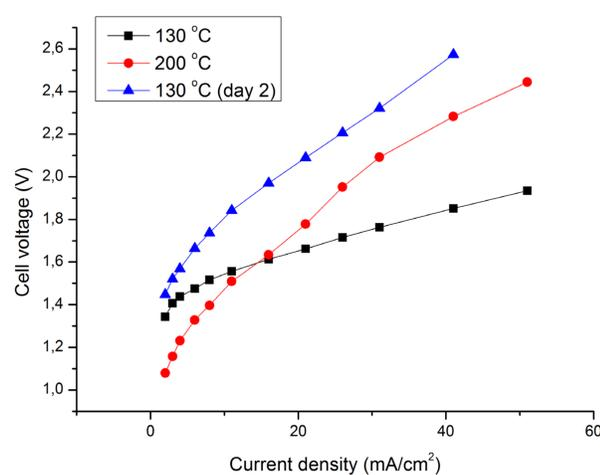
Figure 2: Polarisation curve for electrolysis mode. The cathode had a Pt loading of 0.7 mg/cm<sup>2</sup> and a Nb-P loading of 1.2 mg/cm<sup>2</sup>. The anode had a IrO<sub>2</sub> loading of 2.1 mg/cm<sup>2</sup> and a Nb-P loading of 2.1 mg/cm<sup>2</sup>.
