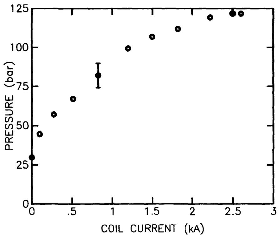
*Fig. II.4. Ethanol peak pressure as function of coil current. Points obtained with 40  $\mu$ l ethanol dose and 2.5 kV charging voltage for the arc discharge capacitor.*
