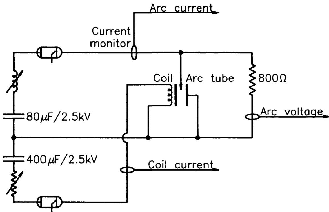
*Fig. III.9. Diagram of power supply circuit for the arc tube and the magnet coil.*
