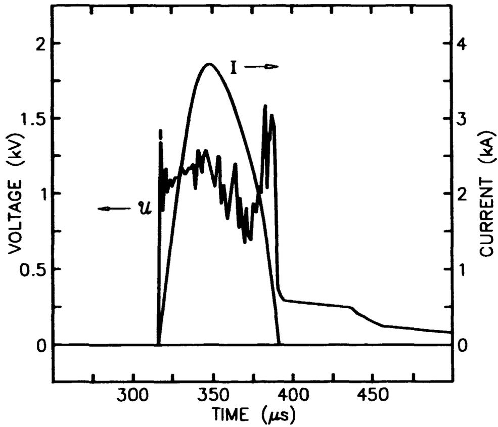
*Fig. IV.4. Arc discharge characteristics for the hydrogen module. Arc voltage (U) and arc current (I) versus time. Same conditions as in Fig. IV.3.*
