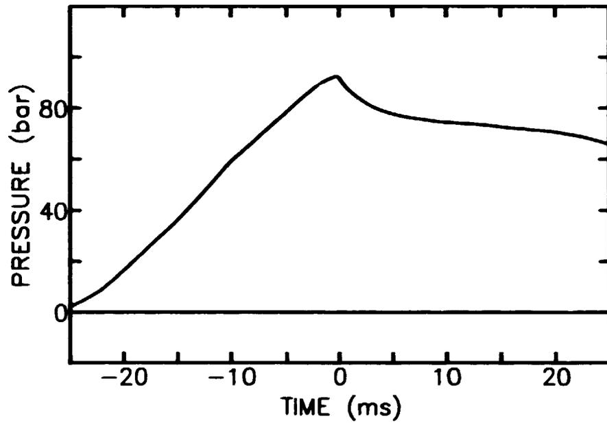
*Fig. III.5. Pressure transient in the rupture disc pressure chamber of Fig. III.3.*
