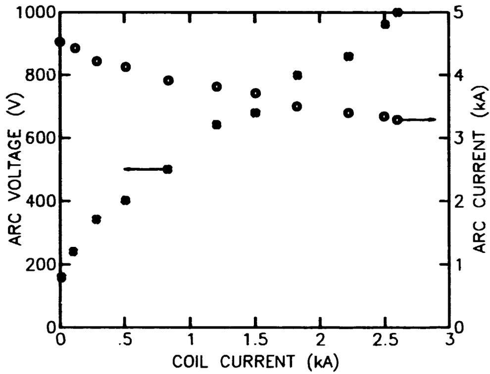
*Fig. II.5. Arc voltage at maximum arc current and arc current as a function of coil current (40  $\mu$ l ethanol, 2.5 kV charging voltage).*
