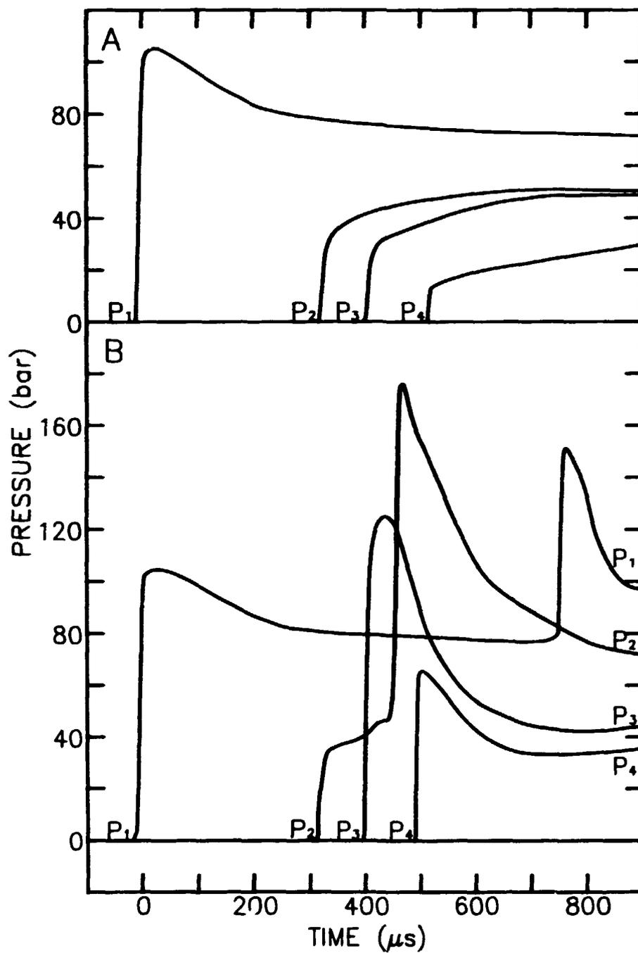
*Fig. III.4. Barrel pressure transients. Signals from pressure probes P1 to P4, Fig. III.3. Upper part (A) from shot without ignition, lower part (B) from shot with ignition of the ethanol arc module. Ethanol dose: 40 μl, discharge capacitor voltage: 2.5 kV and coil current: 2.5 kA.*
