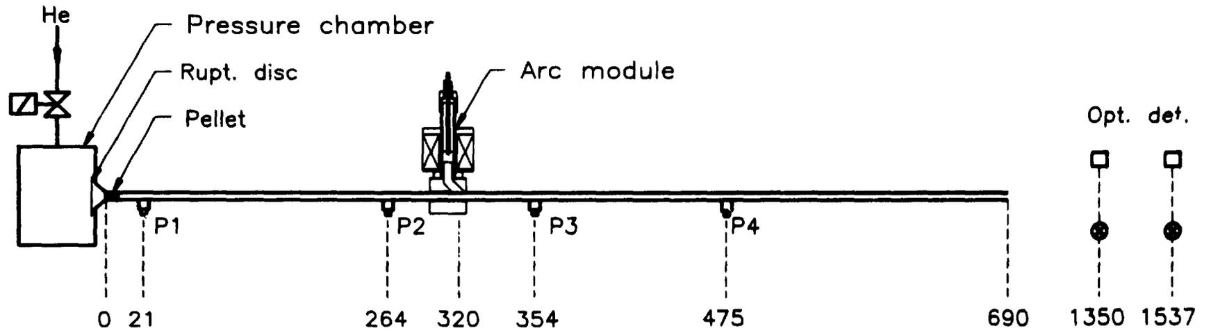
Fig. III.3. Diagram of experimental set-up for acceleration of plastic dummy pellets with the ethanol arc module.
