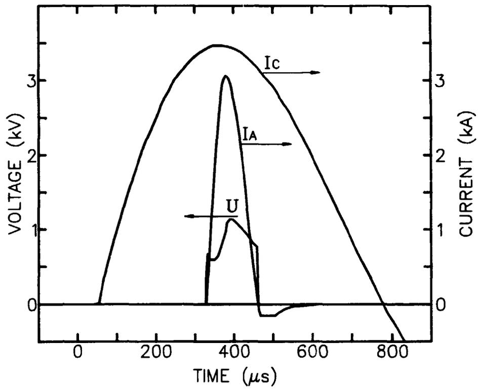
*Fig. III.7. Arc discharge characteristics for the ethanol module. Arc voltage ( $U$ ), arc current ( $I_A$ ) and coil current ( $I_C$ ) versus time.*
