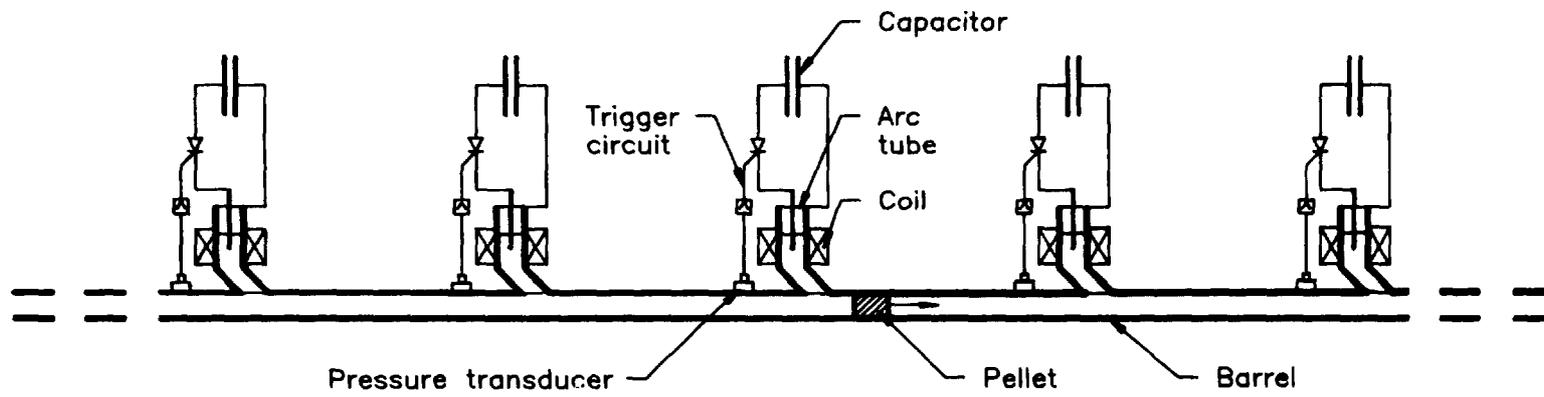
Fig. 1.1. Schematic diagram of multi-stage pneumatic acceleration.
