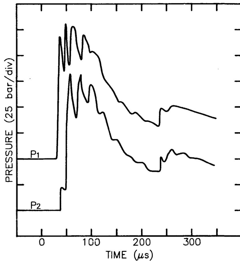
*Fig. II.3. Ethanol vapor pressure transients. Signals from pressure probes P1 and P2, Fig. II.1. Same conditions as for Fig. II.2.*
