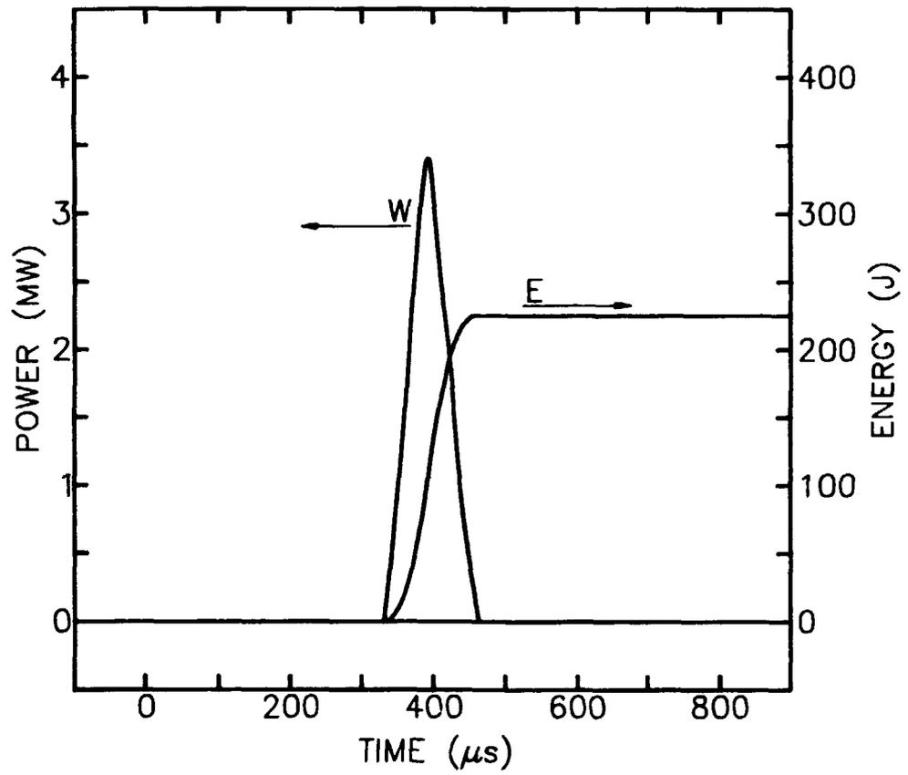
*Fig. III.8. Arc power ( $W$ ) and energy ( $E$ ) versus time for the ethanol module.*
