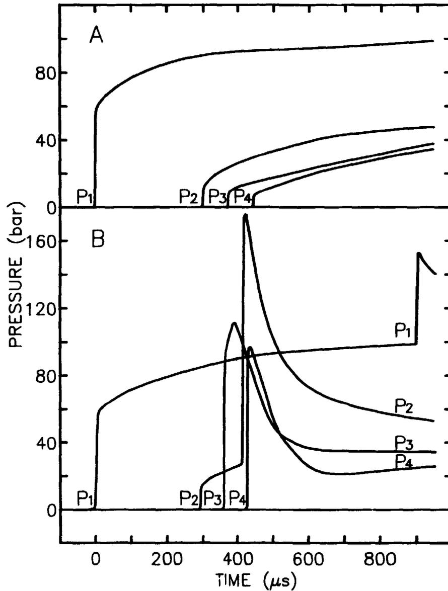
*Fig. IV.3. Barrel pressure transient. Signals from pressure probes P1 to P4, Fig. IV.2. Upper part (A) from shot without ignition; lower part (B) from shot with synchronized ignition of the hydrogen arc module. Hydrogen dose:  $100 \text{ bar cm}^3$ . Peak arc power: 5 MW. Coil current 2.3 kA.*
