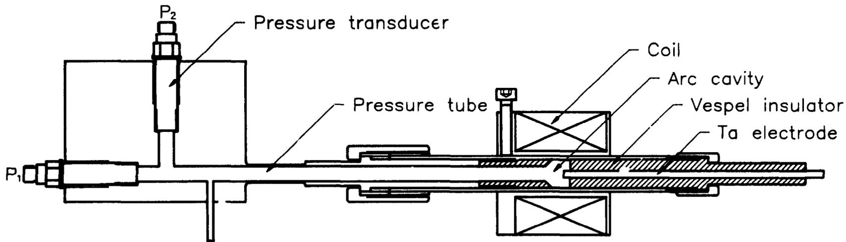
Fig. II.1. Diagram of ethanol arc discharge tube.
