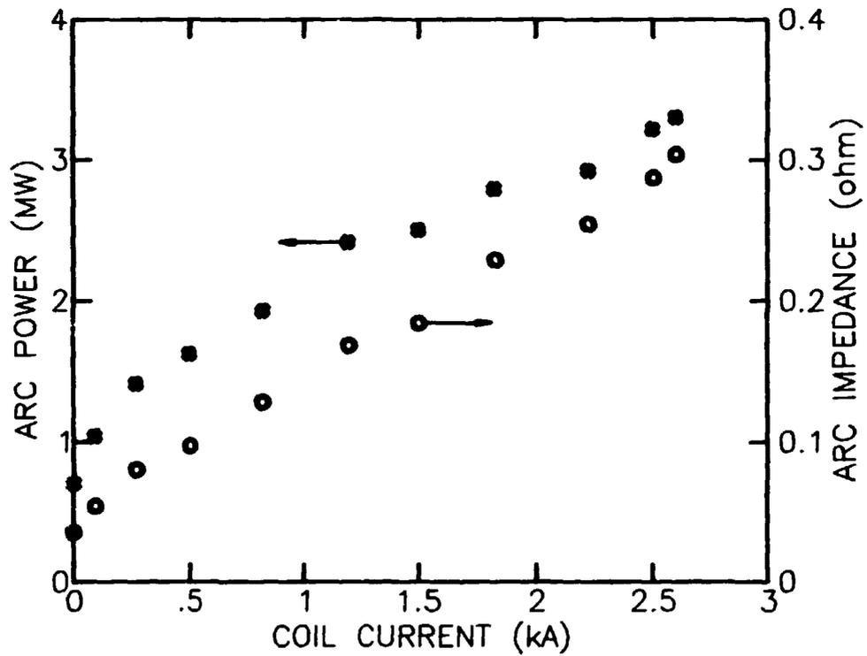
*Fig. II.6. Arc power and arc impedance as a function of coil current. Points calculated from data in Fig. II.5.*
