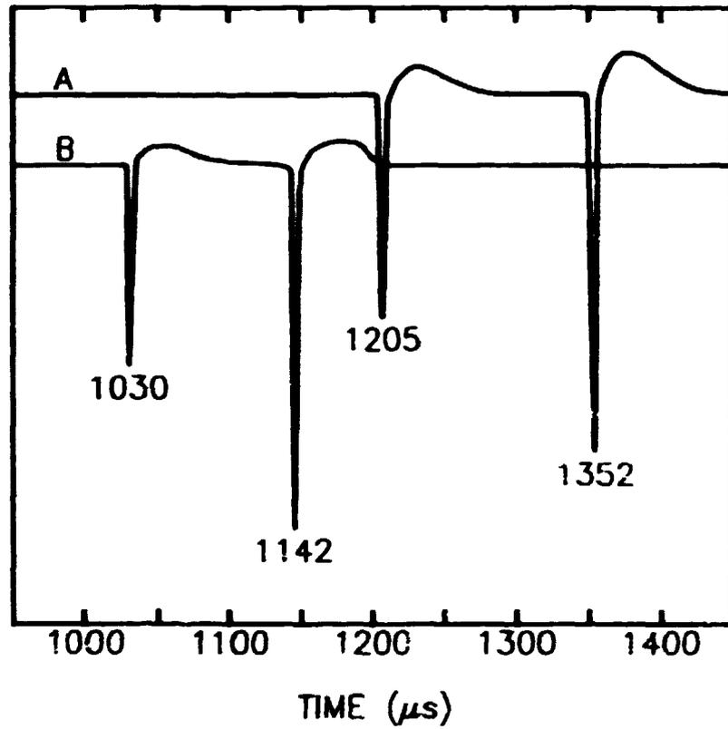
*Fig. III.6. Time-of-flight signals from optical detector. Trace A: without firing of arc module; trace B: with the arc module fired.*
