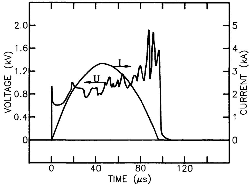
*Fig. II.2. Ethanol arc discharge characteristic. Arc voltage (U) and arc current (I) versus time. Ethanol dose: 40 μl. Coil current: 2.5 kA.*
