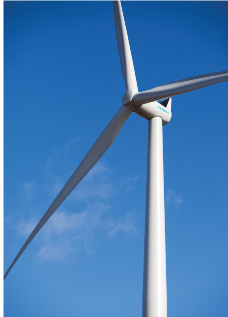
Figure 1.1: Siemens 3.0MW prototype direct drive wind turbine with 101 m rotor.
