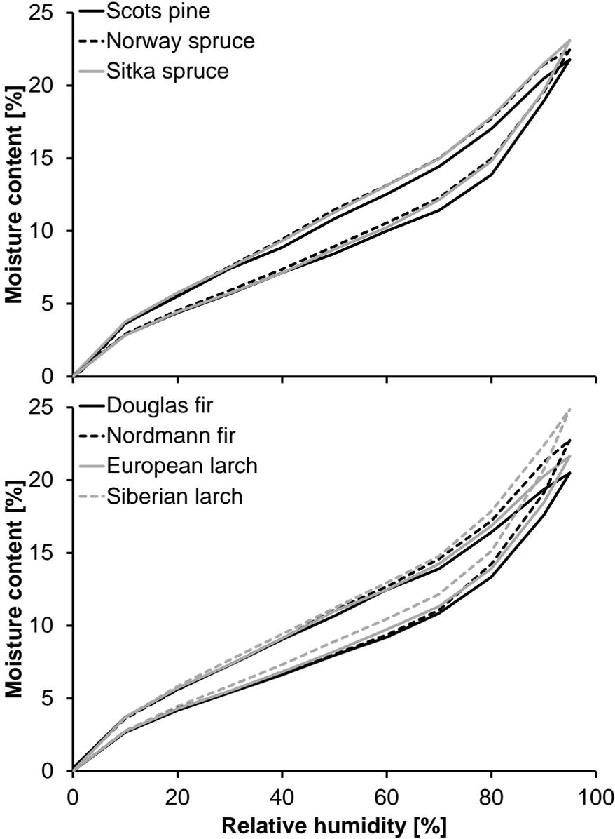
Figure 4: Sorption isotherms for the seven species of softwood. Note that the adsorption isotherm ends at 95 % RH which is the starting point for the desorption isotherm. Thus, the latter is not a true desorption isotherm, but a scanning curve (Engelund et al. 2010).
