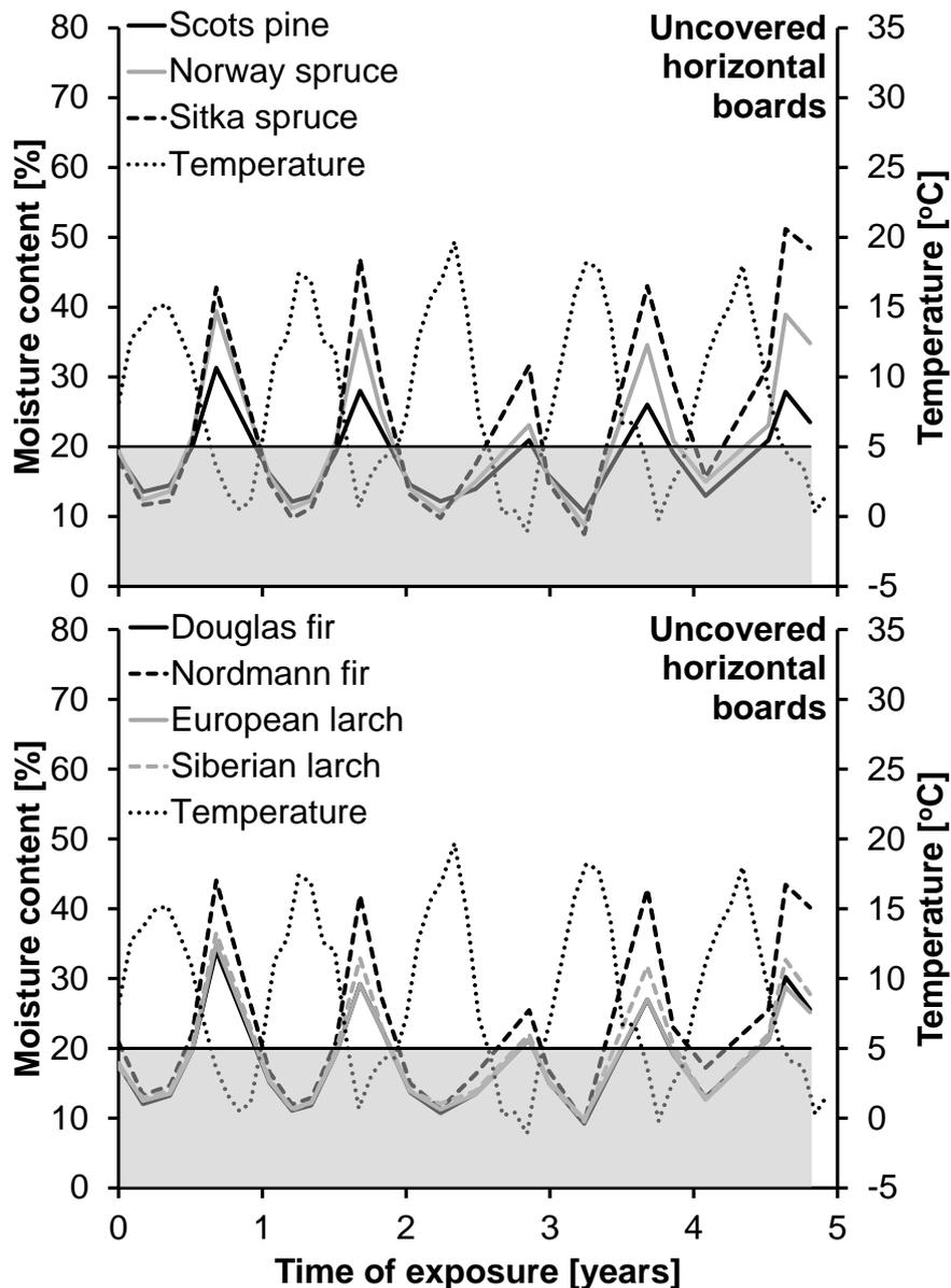
Figure 5: Moisture content and average monthly temperature in the first 5 years of exposure for uncovered horizontal boards (use class 3). Grey area marks region of low risk of biological decay.
