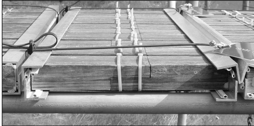
Figure 2: Lap-joints after 3 years of exposure
