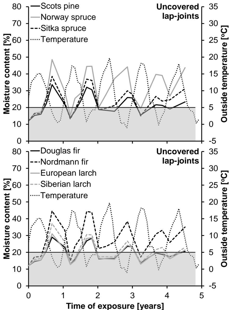
Figure 6: Moisture content and average monthly temperature in the first 5 years of exposure for uncovered lap-joints (use class 3). Grey area marks region of low risk of biological decay.
