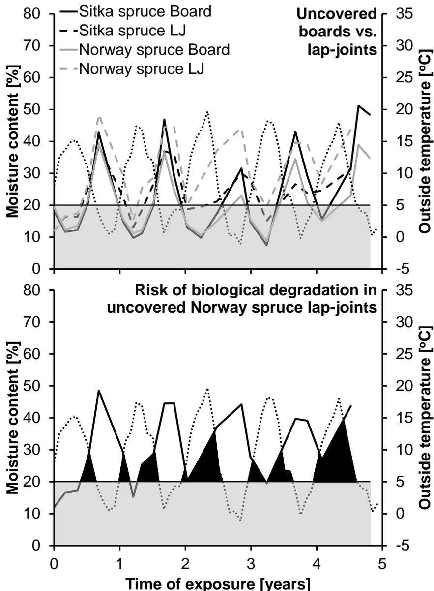
Figure 7: Moisture content and temperature for uncovered boards and lap-joints of Sitka spruce and Norway spruce (top). Illustration of periods of increased risk of biological decay (black areas) in uncovered Norway spruce lap-joints (bottom).
