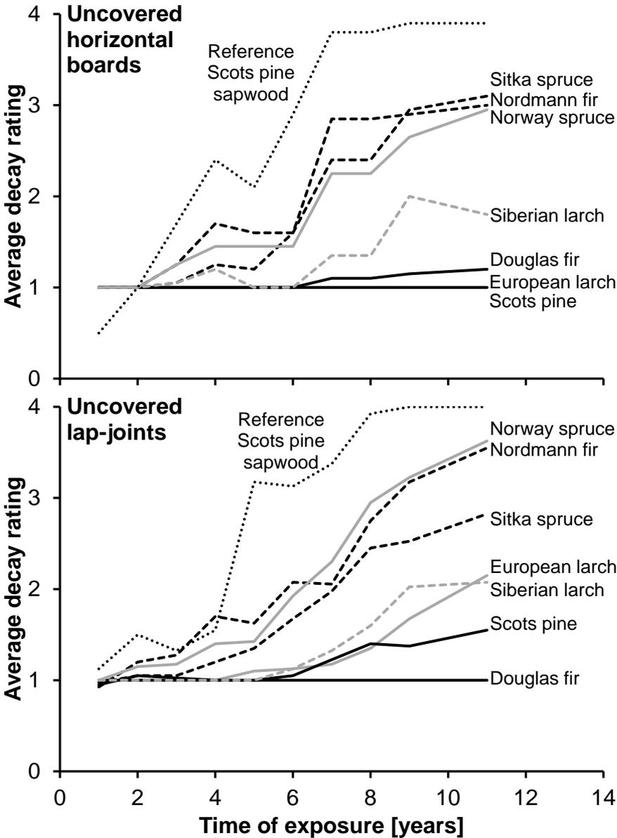
Figure 8: Decay index vs. years of exposure for uncovered boards (top) and lap-joints (bottom).
