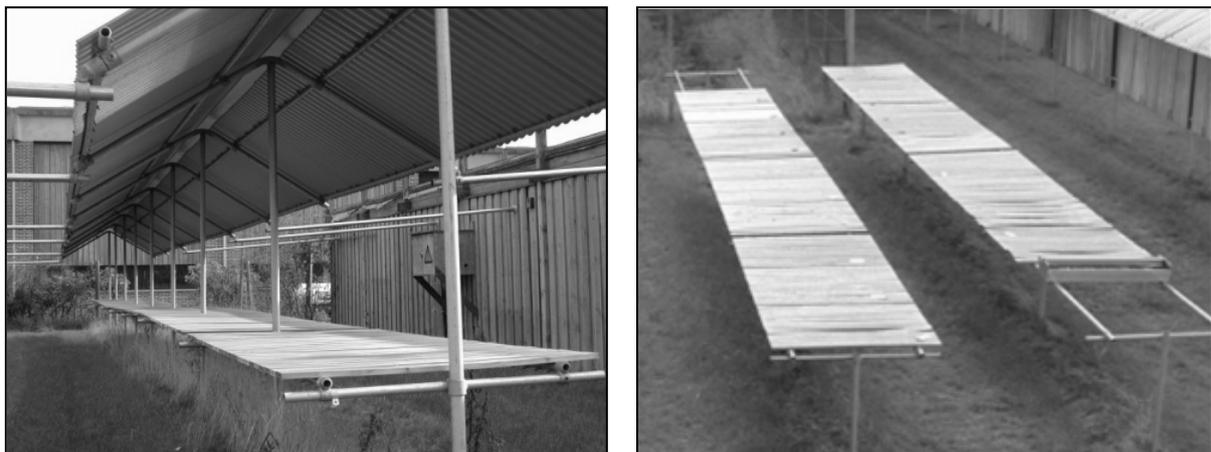
Figure 1: Covered (left) and uncovered (right) boards exposed at the test site.
