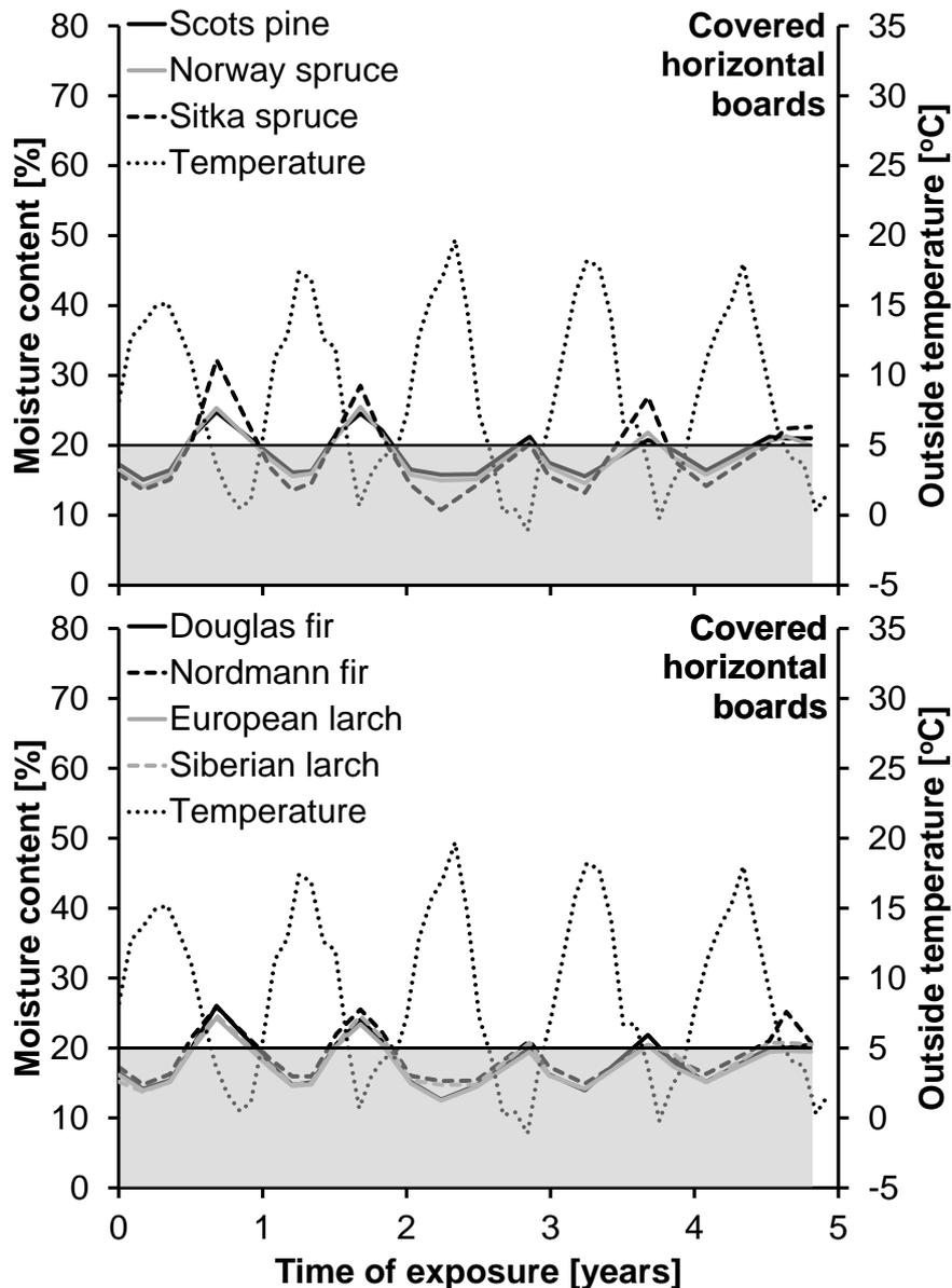
Figure 3: Moisture content and average monthly temperature in the first 5 years of exposure for covered horizontal boards (use class 2). Grey area marks region of low risk of biological decay.
