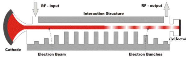
Fig. 1: Schematic drawing of a Travelling Wave Tube
