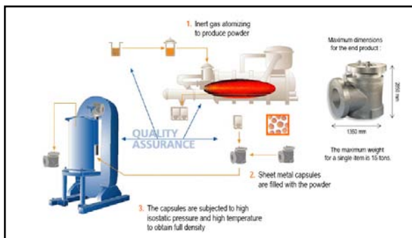
Figure 2 – HIP P/M sheet metal capsule production
