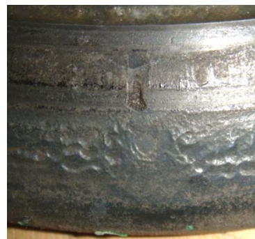
Figure 1 – Local burn mark on spindle seat created by high temperature corrosion
