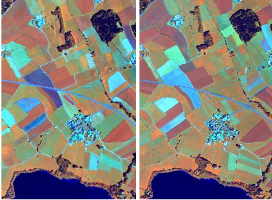
Fig. 1. HyMap bands 27 (828 nm), 81 (1,648 nm) and 16 (662 nm) as RGB, 30 June 2003 8:43 UTC (left) and 4 August 2003 10:23 UTC (right).
