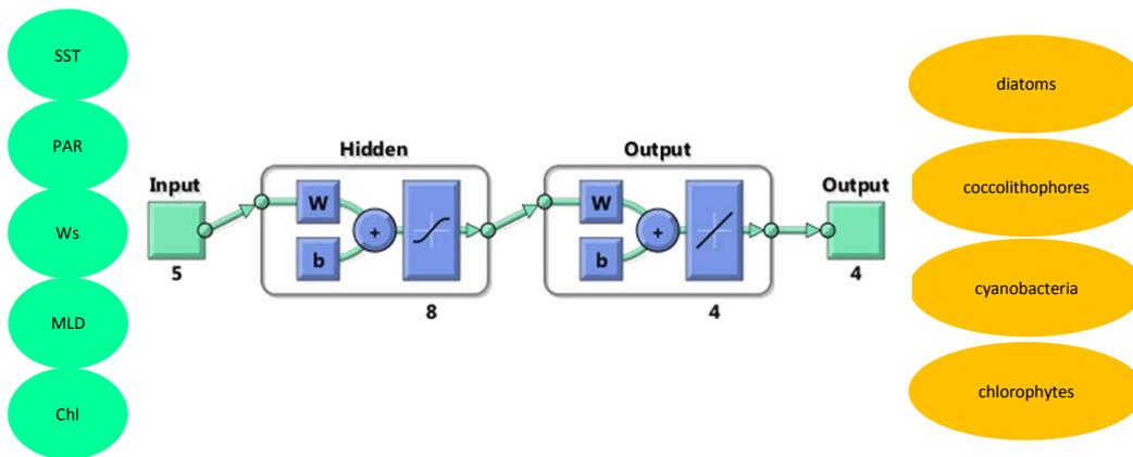
**Fig. 2.** A conceptual model illustrating how the ANN interprets the relationship between input variables, and between input and target variables. Each hidden neuron in layer 1 computes the sum of input values multiplied by connection weights, and calculates the activation value of each neuron (being a nonlinear sum of all inputs). Each output neuron in layer 2 is a linear sum of the activation values from all layer 1 neurons multiplied by respective connection weights.
