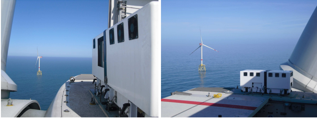
Figure 111: Lidar system (scanner unit and Windcube) on the top of a Repower 5M measuring the inflow.
