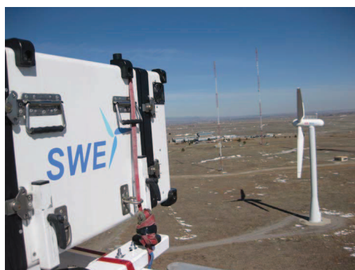
Figure 110: SWE scanner mounted on the CART-2 machine for Lidar Assisted control purposes.
