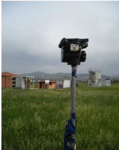
Figure 183: A recent maintenance intervention at the MTP5 radiometer – a microwave source for scanning angle's alignment – (F. Scanzani © 2009 by kind permission of ISAC CNR Rome, Italy))
