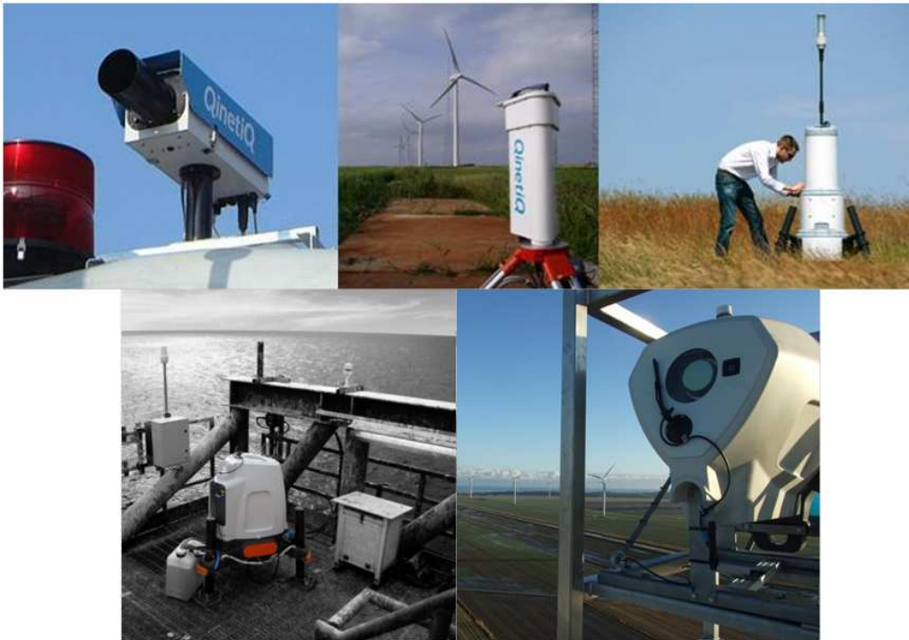
Figure 43: Stages of evolution of the ZephIR lidar. The upper left-hand picture (a) shows the lidar head mounted on the nacelle of a Nordex N-90 wind turbine (March 2003). The top central picture (b) shows a prototype ground-based wind profiler at the Risø wind energy test site at Høvsøre, Denmark. The top right picture (c) shows an early ZephIR production model deployed in the field. The lower pictures show a more recent dual mode ZephIR DM300 deployed on an offshore platform (d) and on a turbine nacelle (e).
