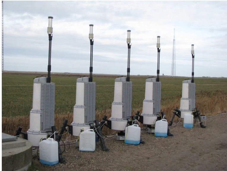
Figure 6: CW wind lidars (ZephIRs) under testing at Høvsøre, Risø DTU
