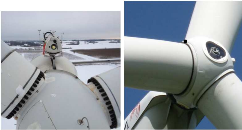
Figure 51: Continuous wave dual mode ZephIR 300 lidars mounted on a nacelle roof (left) and within a wind turbine spinner (right).
