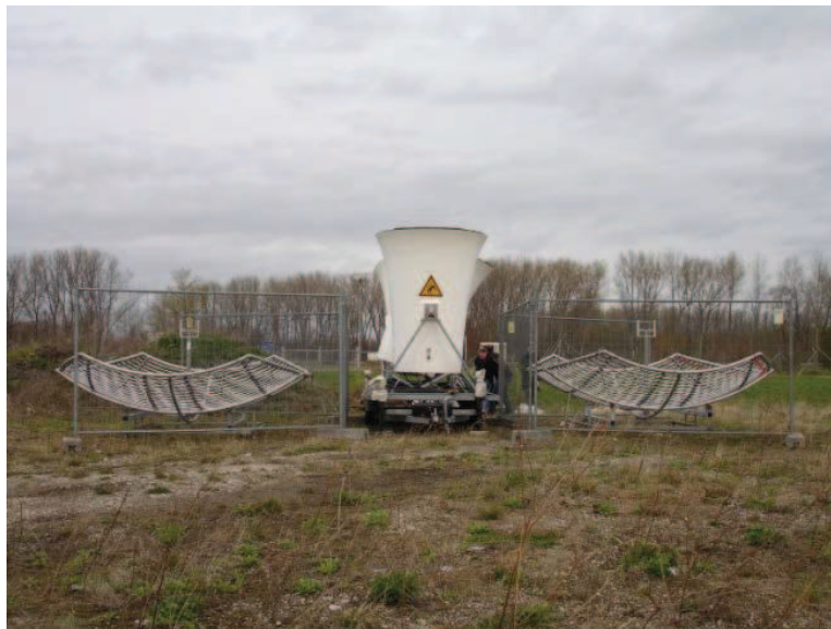
Figure 75: Sodar-RASS. The acoustic antenna is in the middle, the electro-magnetic antennas to the left and right.
