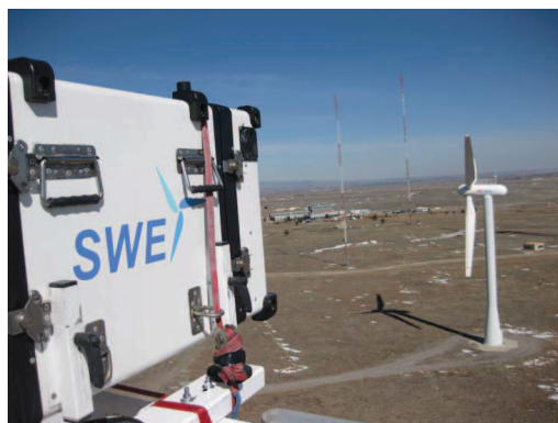
Figure 110: SWE scanner mounted on the CART-2 machine for Lidar Assisted control purposes.
