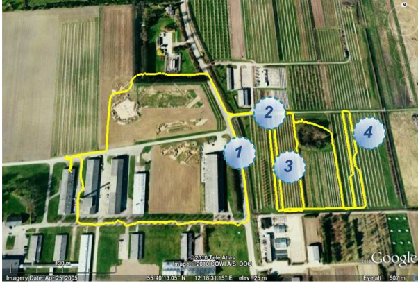
Figure 2: A typical tour covers the track shown in the image as GPS route on Google Earth background. The numbers denote the zones in which the area has been divided for semantic mapping. 1. Open field (Road) 2. Headland 3. Dense trees 4. Sparse trees
