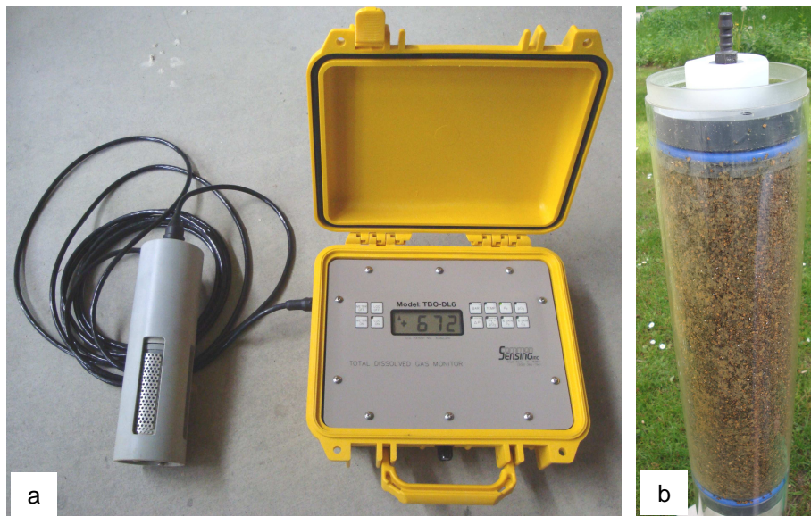
Figure 2.2: (a) A total dissolved gas probe TBO-f (Common Sensing, Inc., Clark Fork, Idaho), and (b) the core sampler developed during the project.
