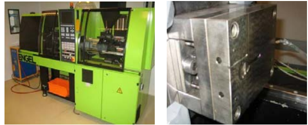
Figure 3: Injection moulding machine used for molding of the plastic parts (left), and the moving side mould with cavity (right).
