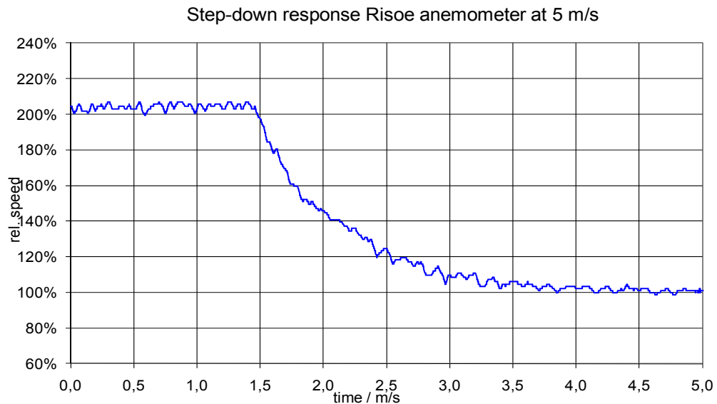
Figure 11.3 Step-down response of Risø P2546 cup anemometer at 5m/s tunnel wind speed.
