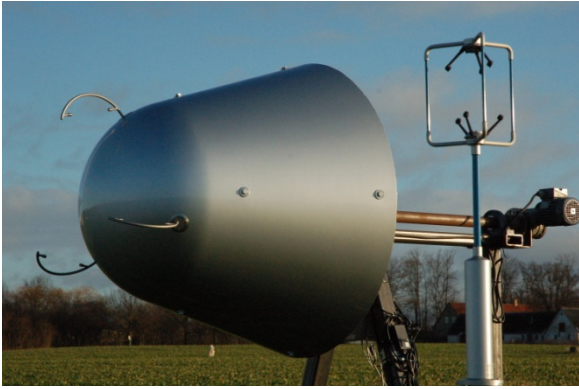
Figure 13.6 Arrangement of the S300 spinner anemometer with "new" sensors in comparison with the sonic anemometer at Risø test site
