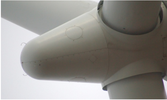
Figure 13.10 The three 1D sonic wind sensors mounted on the 3,6MW wind turbine spinner at Risø DTU Høvsøre test site.
