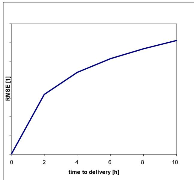
**Figure 14:** The predictability of stochastic wind in-feed is the better, the closer the hour to predict is in time. The forecast error is often measured by the RMSE.
