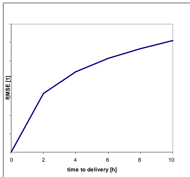
Figure 14: The predictability of stochastic wind in-feed is the better, the closer the hour to predict is in time. The forecast error is often measured by the RMSE.
