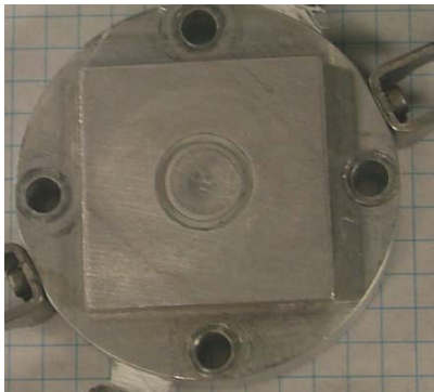
FIGURE 6. Front (beam side) of the fixed degrader after failure, showing barely visible crack in center of the window.
