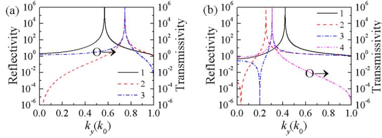
Fig. 3. Reflectivity and transmissivity of a slab. In (a),  $d_1 = 0.1\lambda_0$ ,  $(\varepsilon_{1,e_0}, \mu_{1,\mu_0}) = (-0.3i, -0.3i)$ , and layer 2 is a PEC for curve 1 and of free space for curves 2 and 3. In (b),  $d_1 = 0.1\lambda_0$  for curve 1 and  $d_1 = 0.5\lambda_0$  for curves 2–4,  $(\varepsilon_{1,e_0}, \mu_{1,\mu_0}) = (-0.1i, 0.3i)$ , and layer 2 is a PEC for curves 1 and 2 and of free space for curves 3 and 4.
