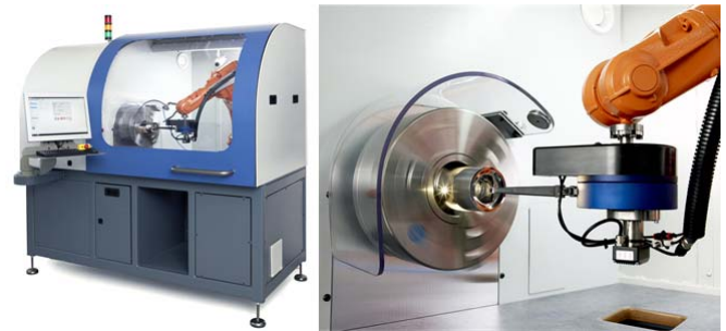
Fig. 1 STRECON's RAP-225 Robot Assisted Polishing machine tool (left); the polishing module close up (right)
