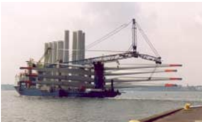
Figure 3 Transport and installation vessel for 160MW offshore wind farm
