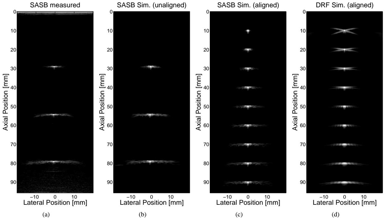
Fig. 4. Visualization of point spread functions using SASB beamforming (a) measured (b) simulated (realistic transducer model) (c) SASB beamforming (compensated transducer model) and (d) DRF beamforming (compensated transducer model).
