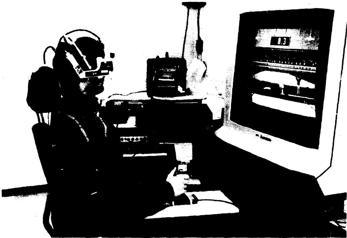
Fig. 3. Automatic recording of eye movements in an experimental session with the 'Gymnastics' video game.
