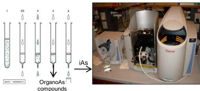
Figure: Steps in the SPE elution procedure for the separation of inorganic arsenic from organoarsenic compounds followed by element-specific detection by HG-AAS
