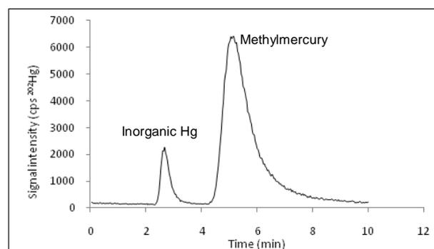
Figure: HPLC-IPCMS chromatogram of the mercury speciation analysis of the CRM DORM-3 (Dogfish muscle), illustrating a nice resolution between the two mercury compounds by the cation-exchange chromatography employed.
