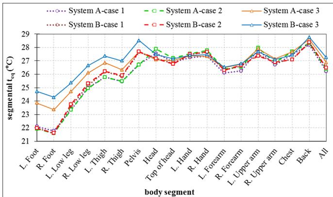
Fig. 4 Equivalent temperature of different body segments of the thermal manikin
